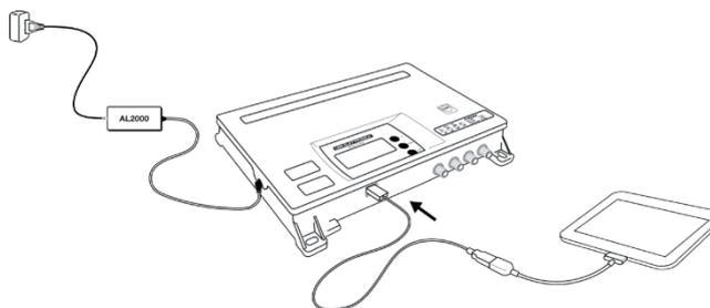
The tablet/smartphone automatically activate the application recognizing the programmable amplifier model.
