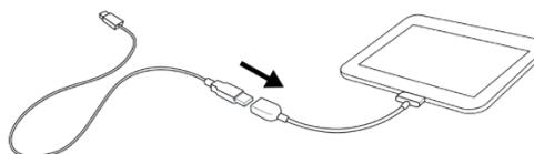
Switth on the tablet/smartphone and connect The cable to AT47SAW.
